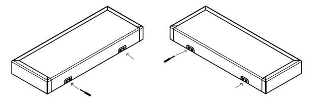
Loosen the screws on the hooks and remove them.
